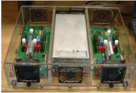
Figure 8. Photograph of the VRM test setup.
